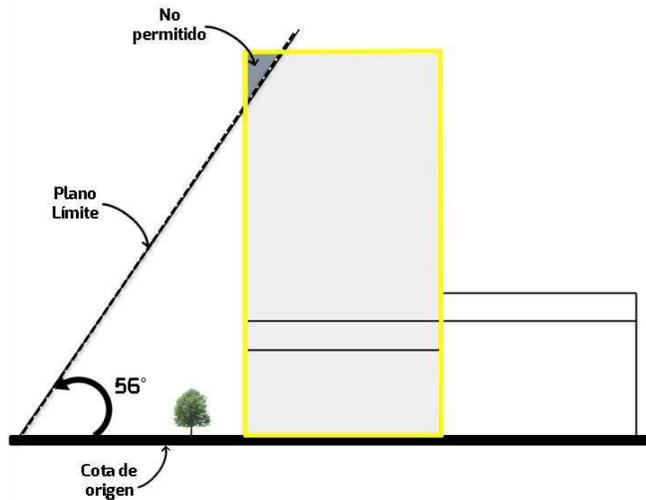
*Aplicación correcta de la Norma. Isométrico y alzado.*
