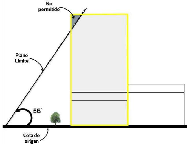
*Aplicación correcta de la Norma. Isométrico y alzado.*
